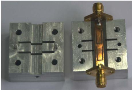
Fig. 9. Photograph of the DBBSF with U-shaped slots.
